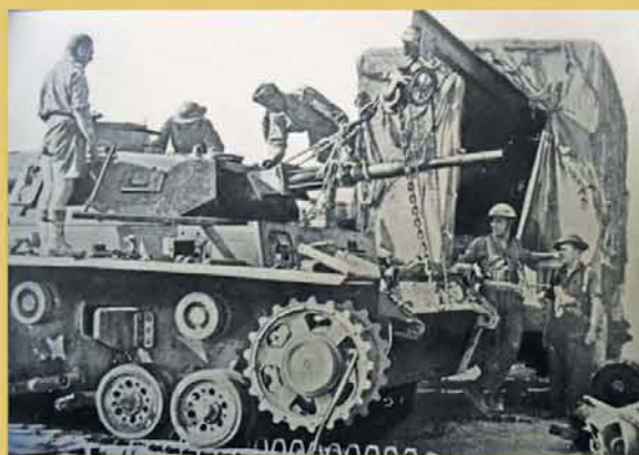
Below: A Retriever Recovery truck being used to remove the gun and Mantlet from a captured German Panzer.
