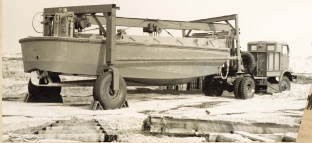
Above: the Seagrave trailer complete with the landing craft is seen here being lowered into the water, ready for operation.
