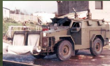
Top left: this Flying Pig spotted at Overlord 2011 was also fitted with the early type of barricade remover.
