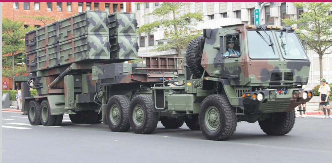
Left: this armoured M1088A1P2 6x6 Tractor Truck was supplied by Oshkosh under Taiwan's Patriot PAC-3 contract, but here it is seen attached to a Tien Kung I surface-to-air missile (SAM) launcher.
