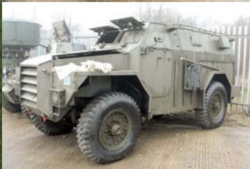
Above centre left: here we see the wireless variant of the Humber FV1600 series truck fitted with the box type body.
