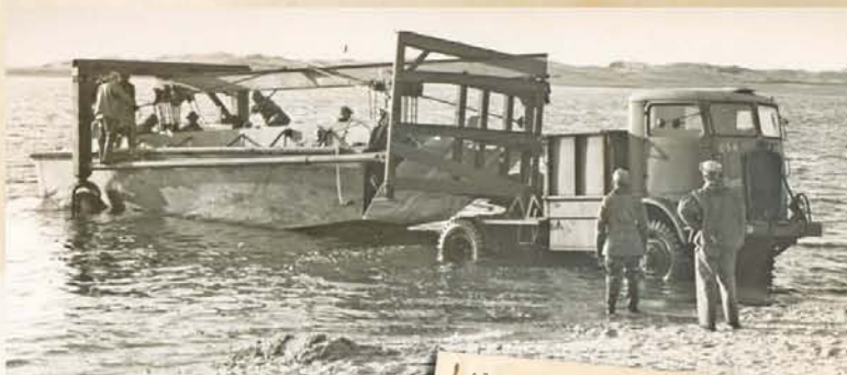
Above: the Seagrave trailer complete with the landing craft is seen here being lowered into the water, ready for operation.
