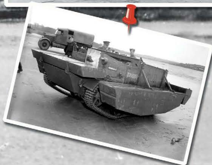
Three images above: here are three Universal Carrier images, one fitted with a wading screen (top right), while the other two are fitted with versions of a kit clearly aimed at enabling the Universal Carrier to swim ashore. I've seen images of the wading screen before, but have to say I've never seen images of Carries fitted with those amphibious kits before...
