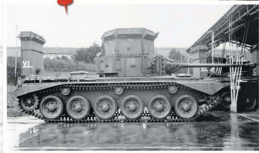
Left: the A34 Comet was probably the best British all-round tank to see service during WW2 and the type remained in service with the British Army until 1960. Shown in this undated image is a Comet fitted with what appears to be a semi-permanent wading/fording kit.
